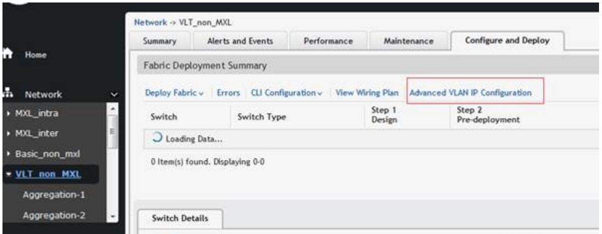
Figure 17. Layer 3 with Resiliency (Routed VLT) with VLT option + Advanced VLAN IP Configuration
